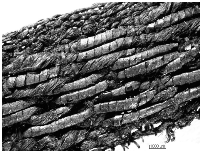
Fig. 7. Silk tabby band with a pattern warp of metal thread found in a grave inside Tartu Cathedral (TM A-172: 231a). Photo by Riina Rammo.
