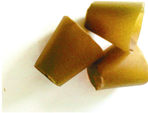
Fig. 4. Plant pots prepared from a composite based on starch and rapeseed cake.
