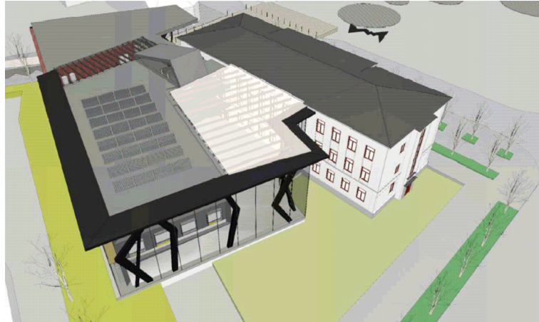
Fig. 1. View on the Rakvere nZEB from south; the cold atrium is fully glazed and the roof window of the warm atrium, dividing the offices to south and north parts, is also seen. The nZEB is connected to an existing building.
