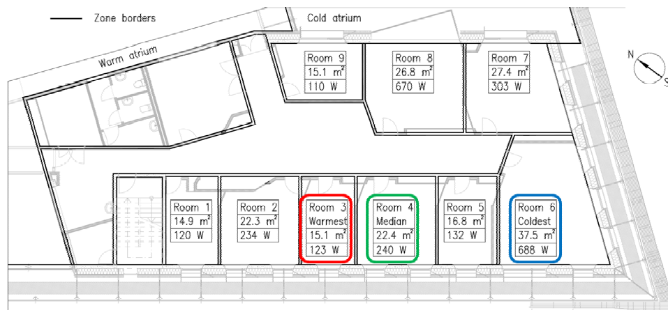
Fig. 2. Office rooms's plan, where the zone borders were slightly simplified compared to architectural solution (depicted in grey).
