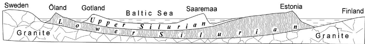
Fig. 2. Ideal geological section of the Silurian formation across the supposed Palaeozoic depression from Sweden (Kalmar) to Finland (Vyborg) after Schmidt (1881).
