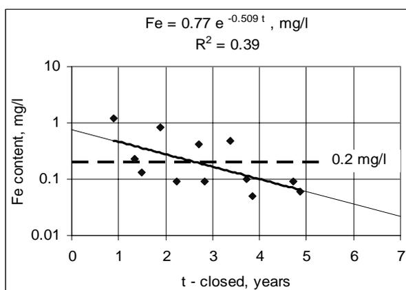
Fig. 3. Decrease in the content of  $\text{SO}_4^{2-}$  and Fe in closed mines.
