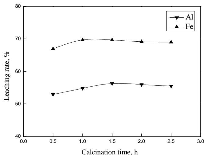
Fig. 7. Influence of calcination time of circular retorting semicoke on leaching rates of Al and Fe.
