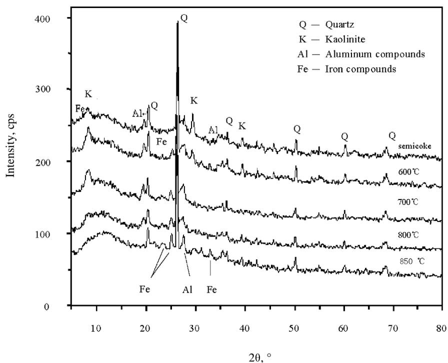
Fig. 1. XRD chart of circular retorting-derived residue calcined at various temperatures.
