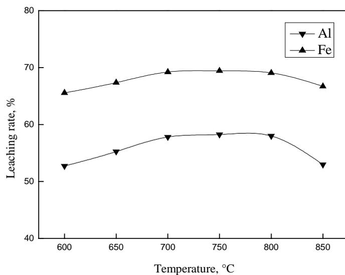
Fig. 4. Influence of calcination temperature of circular retort semicoke on leaching rate of Al and Fe.
