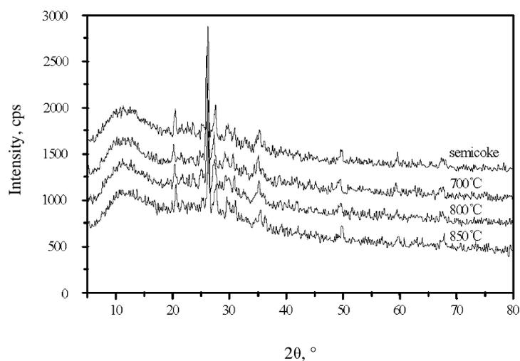
Fig. 3. XRD chart of ash from cogeneration plant calcined at various temperatures.
