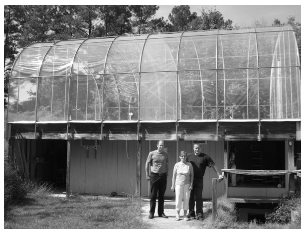
Fig. 2. The dual outdoor Teflon Film smog chamber of UNC at Chapel Hill, NC, USA.
