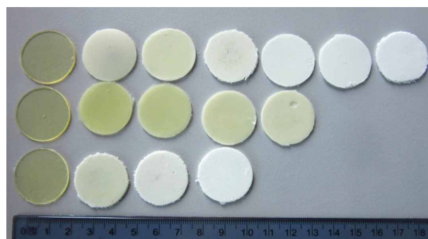
Fig. 1. Samples for thermal conductivity measurement: HGM/epoxy composites (top row), aerogel/epoxy composites (middle row), HGM/PMMA/epoxy composites (bottom row).
