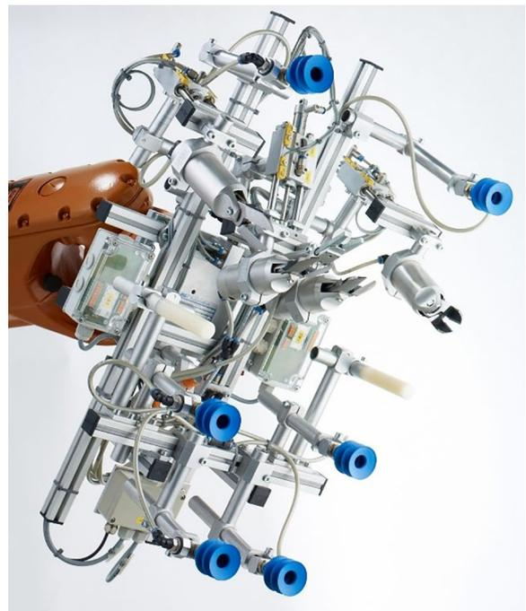
Fig. 4. End of arm tooling [8].
