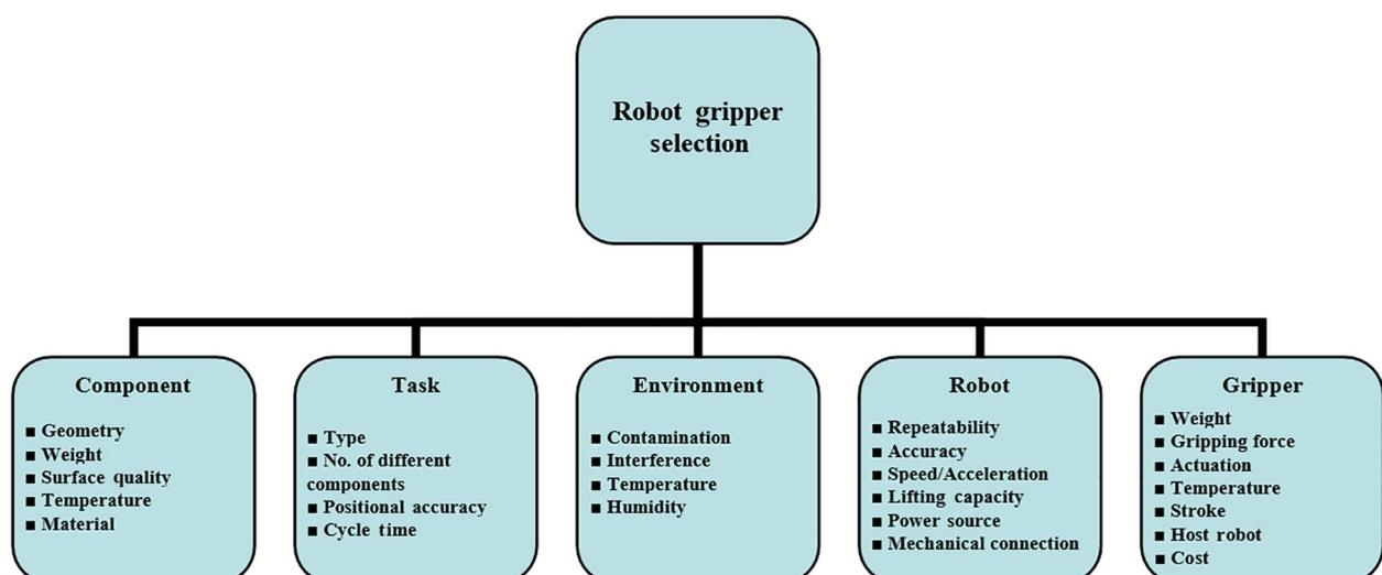
Fig. 5. Governing factors for gripper selection (adapted from [2]).
