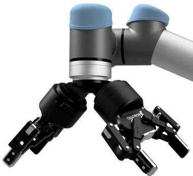
Fig. 3. Multiple gripper frame [7].
