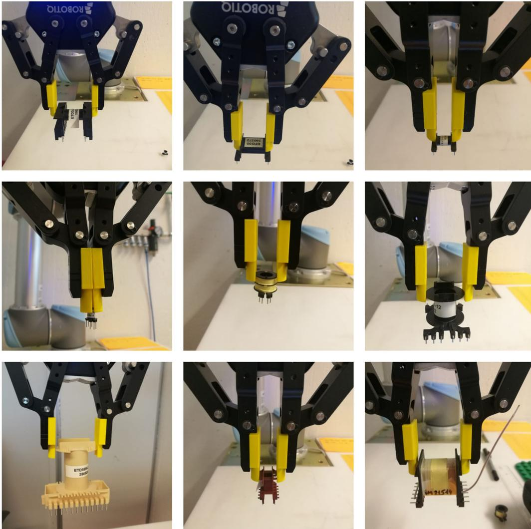
**Fig. 9.** Universal gripping for the use case using finger modification method.
