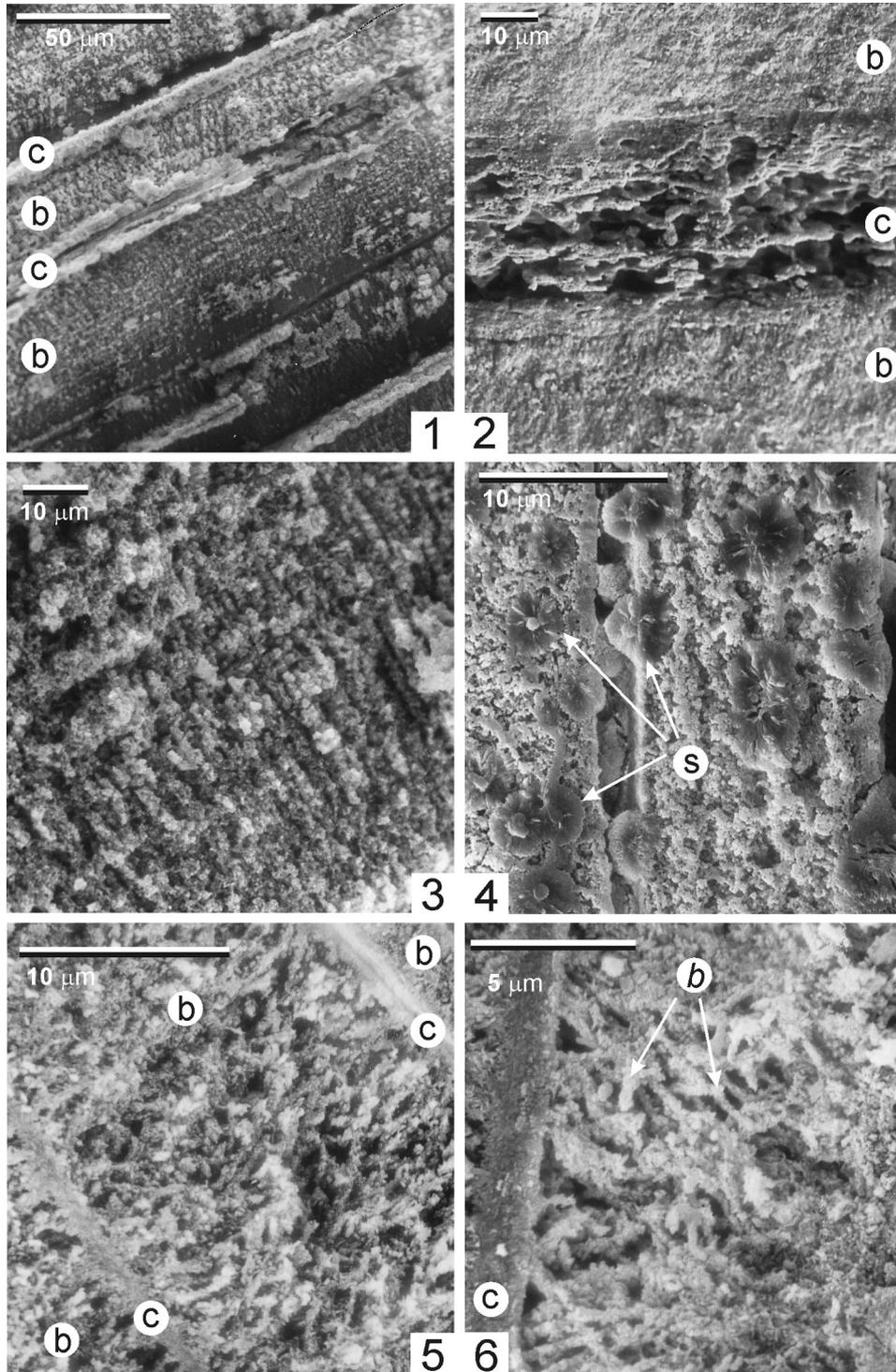
zation of the organic compound in baculate laminae. This second generation of apatitic matter inside shells has a characteristic structure and has been termed as collophanous calcium phosphate (CCP) by Holmer (1989).
